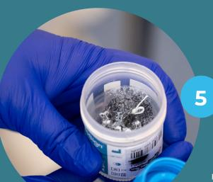
The sponge is put in a lab container, the thread removed, the container sealed, and sent to our laboratory for testing.
